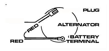
You will hookup the large wire to the 'bat' terminal of the alternator and run the other end to the starter solenoid or wherever your positive battery cable attaches to. Install the sleeve & ring and connect it to the battery cable post of the starter solenoid or wherever your positive battery cable attaches to.
