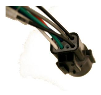
If you have an 91-93 Mustang 5.0 MANUAL TRANS OXYGEN SENSOR HARNESS, it should be pinned like this. Be sure to pin your new harness like this:
