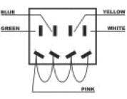
Blue: Splice to the right front turn signal wire. White: Splice to the right rear turn signal wire. Yellow: Splice to the left rear turn signal wire. Green: Splice to the left front turn signal wire. Pink: Connect to the emergency flasher. The flasher should be connected to a "fused" battery feed circuit.
