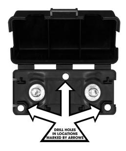
To remove the splash resistant cover, press the front cover clip and lift the cover. Under the cover are two 8 millimeter studs with nuts installed for mounting the Mega fuse and wire cables. NOTE: This unit is designed to accept one Mega fuse and two 5/16 ring terminals. Only use number four to eight wire gauge wire when making wire cable connections to this unit.
