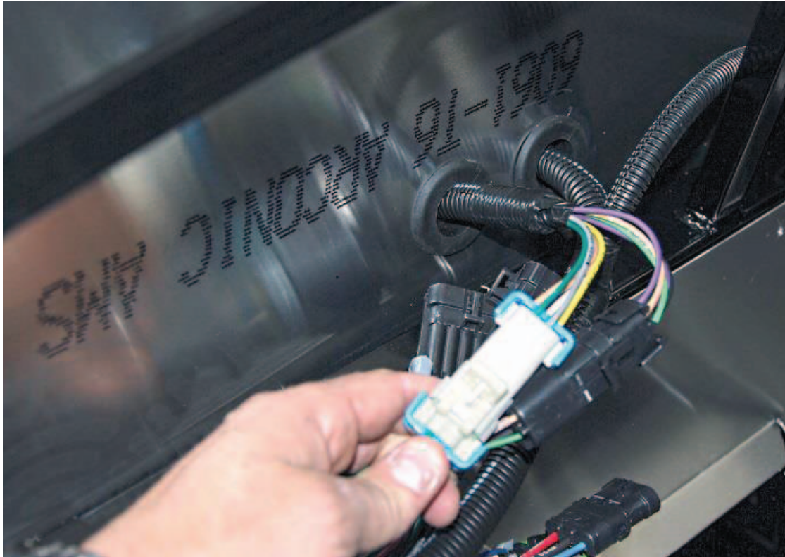
Connect the rear harness connectors to the connectors on the main harness.
