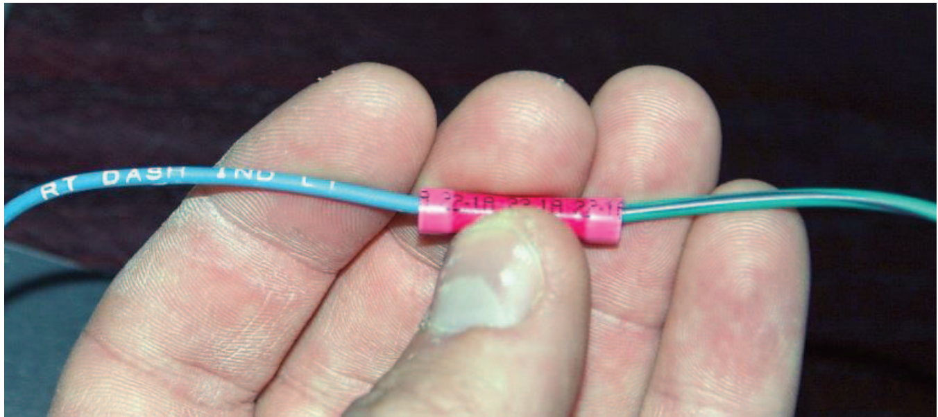
Connect the blue right turn indicator wire to the gauge green/red wire.
