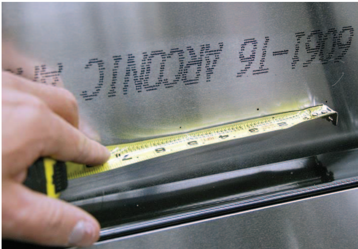
Measure left from the first point and mark the firewall at 2.50" and 5.00" so there are three marks altogether.
