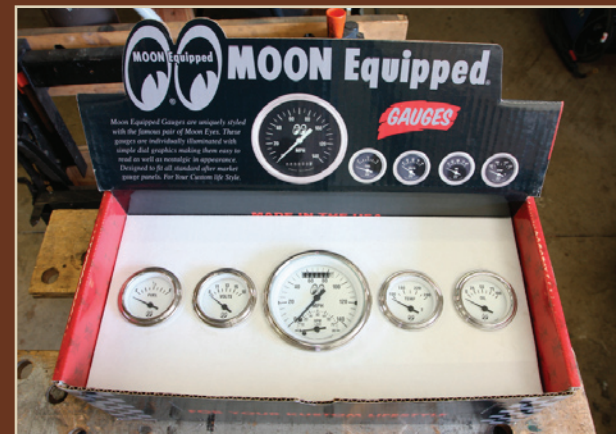
We'll be using a five-gauge white face set of Mooneyes gauges made by Classic Instruments for the Willys. The set features a 3 3/8-inch electronic speedo/tach combo while the other four gauges are 2 1/8-inch and monitor fuel level, water temperature, volts, and oil pressure.
