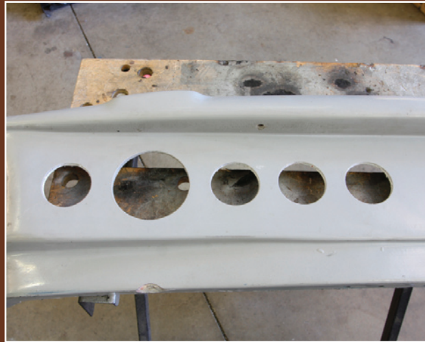
Once the holes were drilled, a file was used to deburr all the edges; fiberglass splinters are not fun!
