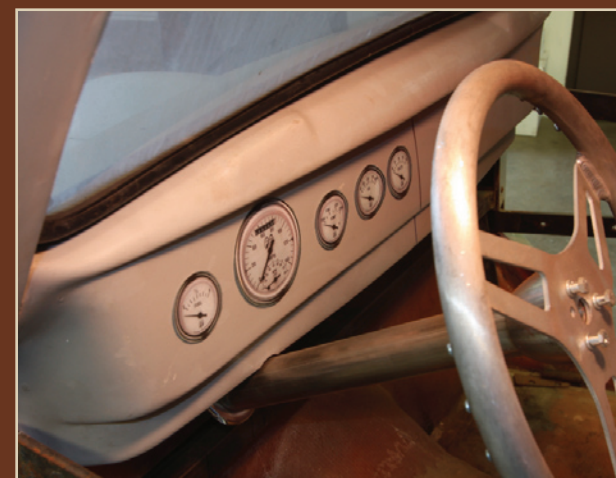
One of the tricks we used in figuring out how we wanted to layout our gauges was to scan the faces and print them out. Once cut out, we taped them in various layouts to find the one we liked the best.
