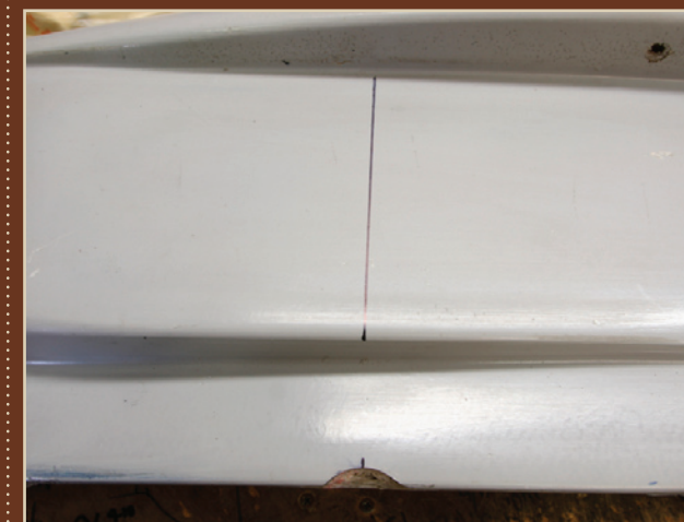
Since the speedo/tach gauge will be centered over the column, we'll start there. The dash already had a small relief made to clear the column so finding the center was pretty easy.
