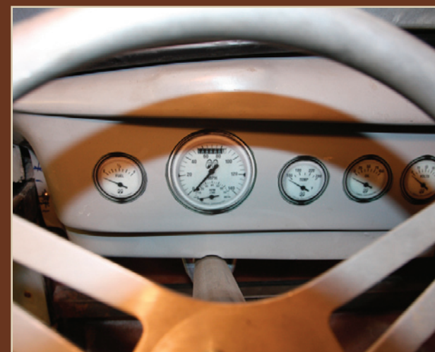
We opted to center the speedo/tach combo over the column with the fuel gauge on the left and the trio of engine vital gauges on the right.
