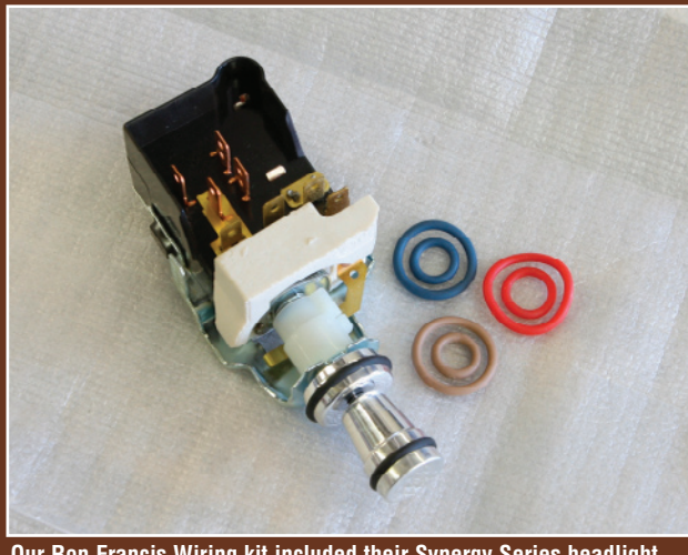
Our Ron Francis Wiring kit included their Synergy Series headlight switch which includes the four different colored accent rings; black, tan, red, and blue.
