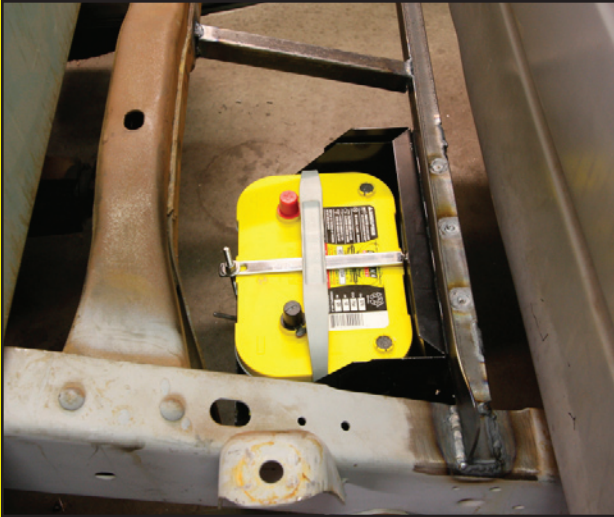
Safe and secure, the new Optima battery is held in place with the hardware provided.
