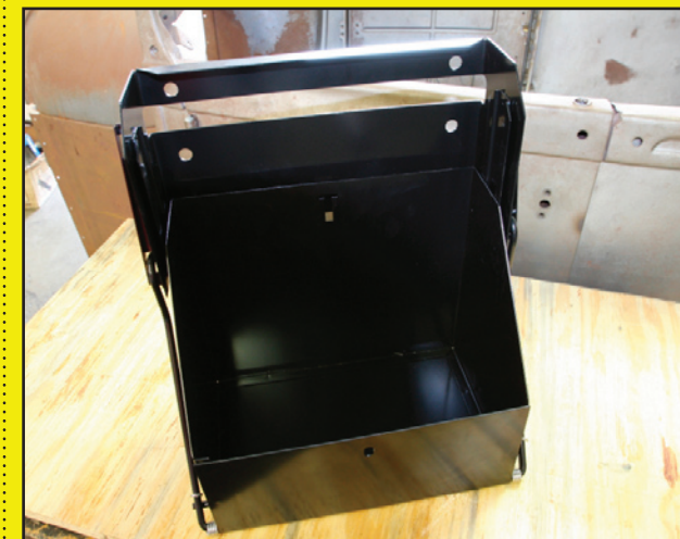
By releasing a pair of spring-loaded latches, the battery box drops down in its mount 4¼ inches. The battery box can also be completely removed from its mount.
