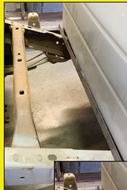
The best spot to hide the battery was to hang it off the framerrails under the bed; the obvious problem then becomes access.
