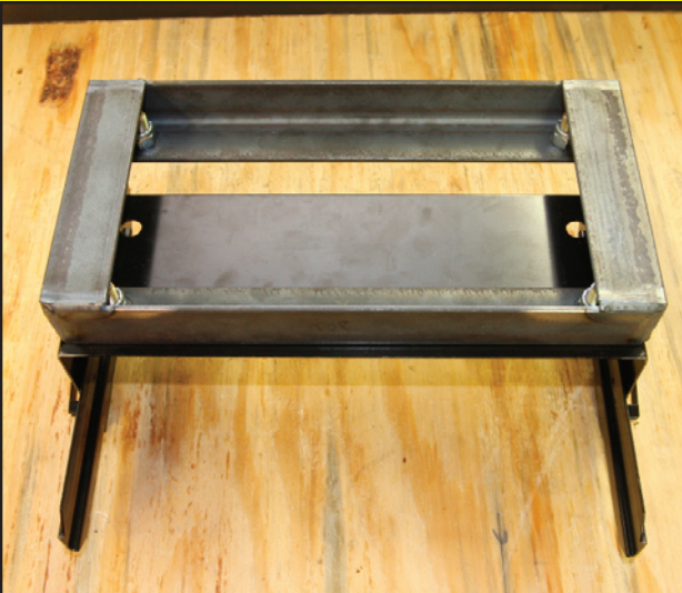
The mount for the battery box then bolts to the framework.
