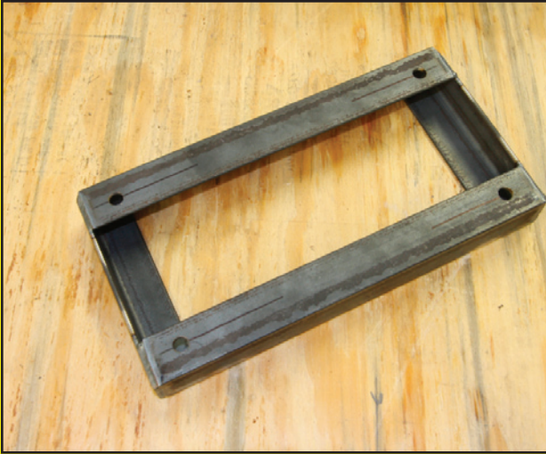
This framework will be welded to the mount that has been attached to the frame.
