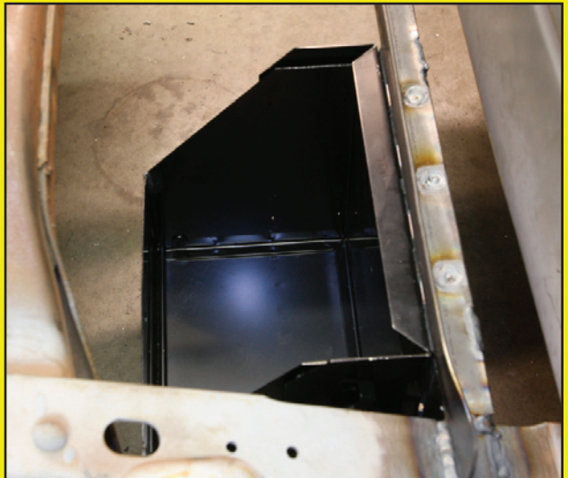
Finally, the drop-down mount and the box is bolted in place.
