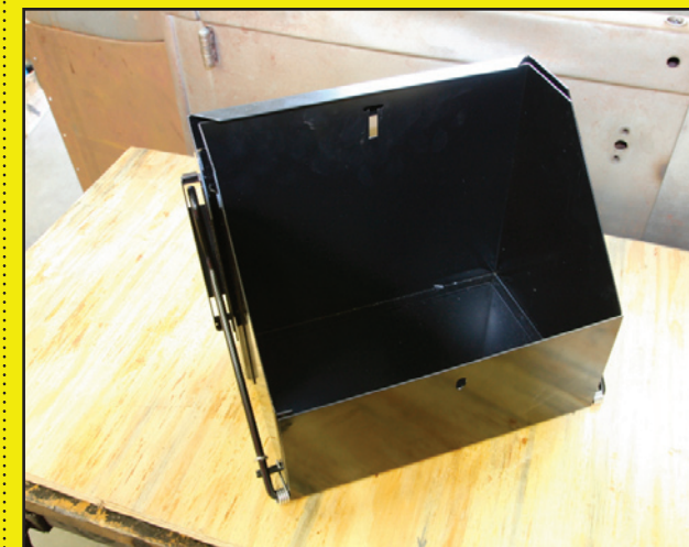
Here's the drop-down battery box from Speedway Motors, here it is in the installed, or raised, position.
