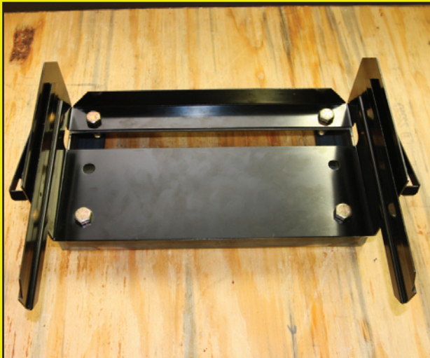
Viewed from the battery box side, the mount has been attached to the previously shown framework.
