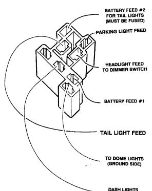
The battery feed #2: is a 12 volt, hot all the time <u>input</u>. Run a wire from a fused source at the fuse block to feed this connection. This wire must be fused to protect the tail light circuit.
