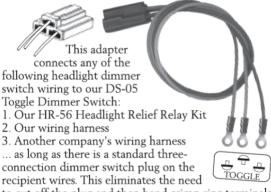
to cut off the plug and then hand crimp ring terminals for attaching to the toggle dimmer switch. The blue wire is the feed wire, which will go to the center terminal on the toggle, red is low beam and brown is high beam.
