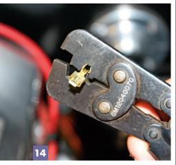
Ron Francis supplies the F-crimp connectors needed to complete the install, which look like regular spade connectors, but require a special Delphi Packard crimper tool, crimping the wire separately from the insulation.
