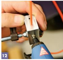
Probably owing to my choice of wiring route, the coil wire was too short to reach the HEI distributor, and hence required lengthening. As the joint would be under the car I used this neat little kit from SpliSeal to make a watertight connection. The wires were spliced together and the joint placed in the aluminum block/mold provided. The two halves damped together and then a heated injection gun was used to fill the block with molten polymer.
