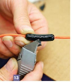
Removed from the mold and the spur cut off, a permanent weather-proof joint is the result.
