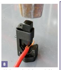
While the terminals at the battery ends of the positive and negative cables were attached using regular terminals with set screws to connect the cables, the other ends required terminals that would bolt to the starter motor (+) and the chassis (-). This tool correctly crimps the terminals to the stripped cable with a single hammer blow. Heat shrink will cover the crimped section.
