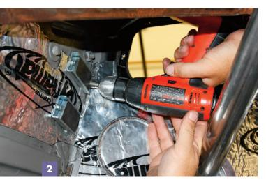
The first step was to install the magnets that hold the fuse panel in place. The picture's not upside down, you're looking up under the dash, where I elected to install the fuse panel. Check clearance behind the panel before drilling.
