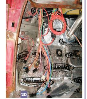
Here you can see the wires for each section or circuit, hanging from the fuse panel (via the line clamp), each with a plastic terminal block. One by one each section is wired. Wires that weren't to be used immediately but may well be wanted in the future (such as a stereo in my case) are coiled and cable tied neatly.
