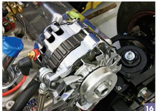
Powermaster supplied the alternator, a CS130style 140A one-wire version. Depending on the current draw requirement of your car. you'll have to decide on the output of the alternator required, by adding up the draw each component is rated at. There's a useful chart on the Powermaster website to help determine this.
