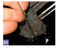
Difficult to see I know, but this is the top of the A-pillar. I ran the interior light wire up this pillar and along the top of the door aperture, to the dome light. A simple trick to assist pulling the wire through a pillar is to feed a length of welding rod down the pillar, then tape the wire to it and pull it back through.
