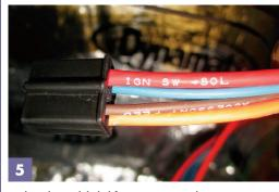
With each wire labeled for its exact use, plus many of the connections pre-assembled, such as this plug for the ignition switch, the chore of wiring is greatly reduced. In fact one of the hardest parts of the job is deciding where to route all the wires!
