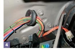
I chose not to use what the instructions referred to as the target (a split metal plate with a large hole, supplied in the kit), but recognizing the need for something similar, I used this large P-clip to route all the wiring through.
