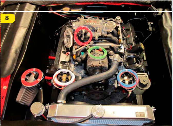
After routing the injector wiring through the firewall grommet and towards the rear of the car, it was decided to "pre-stage" each wiring bag on its input/output device. Seen here are the wire bundles for the coil packs, MAF sensor, throttle position, and more plugged in and ready to be routed.
