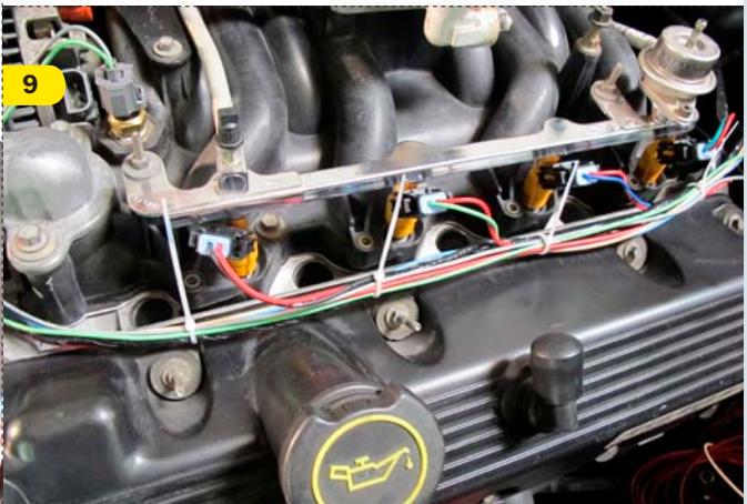
Routing these bundles of wires rearward on the engine while following the initial run from the fuel injectors makes it easy to bundle the wiring together. For now, we're using "sacrificial" tie-wraps to keep things neat and Rusty will be covering the wiring with split loom later once the chassis wiring and any other wiring is integrated into the vehicle.
