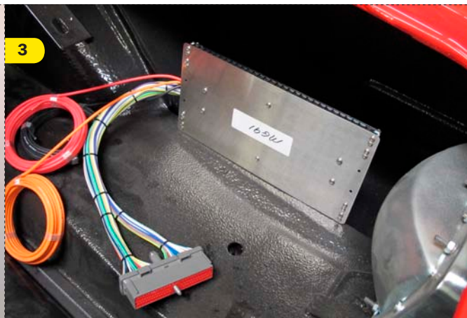
When using a system like this, it is critical to determine your panel location first, with wire routing a secondary but still important consideration. Rusty decided on the right rear trunk area. A trunk block-off panel will be fabricated with the wiring panel mounted on the back of it as mocked up here.
