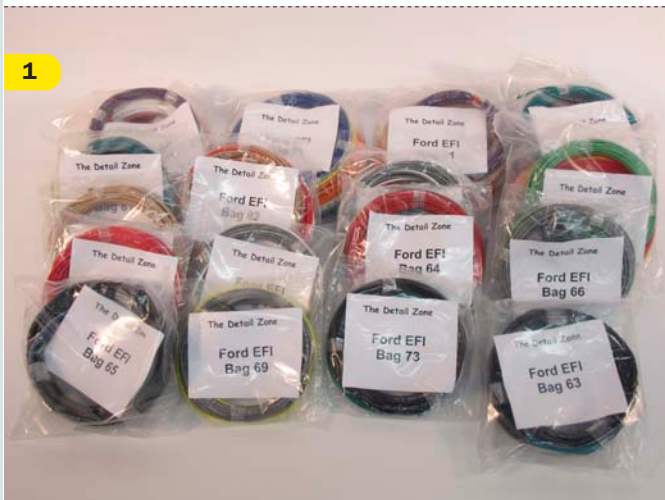
Depending upon the system and options ordered, the panel ships with prepackaged wiring components that are numerically labeled. It makes it super easy, as the instructions tell you which bag to grab next.
