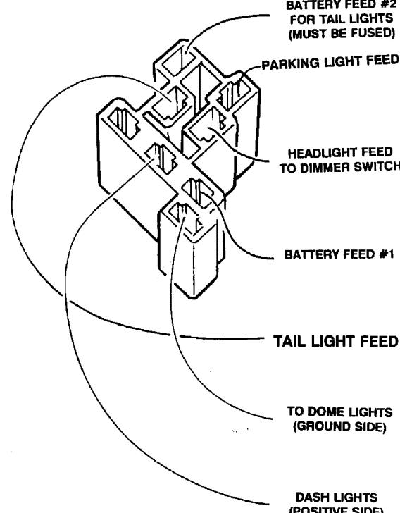
The battery feed #2: is a 12 volt, hot all the time input. Run a wire from a fused source at the fuse block to feed this connection. This wire must be fused to protect the tail light circuit.
