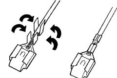
A minimum of 14 gauge wire should be used when wiring the head light circuit and 16 gauge for the tail light circuit. 18 gauge may be used on the dome and dash light circuit.
