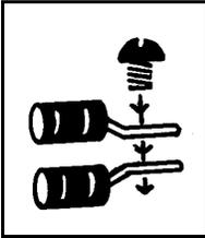
Always put the first terminal under a screw with the fat wire side down as in the drawing. Install any second terminals just the opposite as this will allow the screw to hold squarely and tight. The insulation from one terminal should not interfere with the one next to it.
